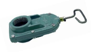
Eclipse Blast Gates are sturdy, inexpensive manual control valves for use with low pressure air up to 5 psig. Accidental shut off is prevented by an adjustable locking device on the handle rod. This lock allows the minimum setting to be fixed at any point.
